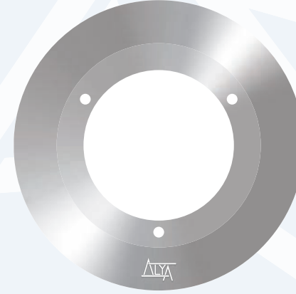
Dairesel Bıçak/Circular Knife 81.25x32x1mm, Çift Bileme/Double Bevel, 3x4.3mm Delik/Hole, 420 Paslanmaz/Stainless
